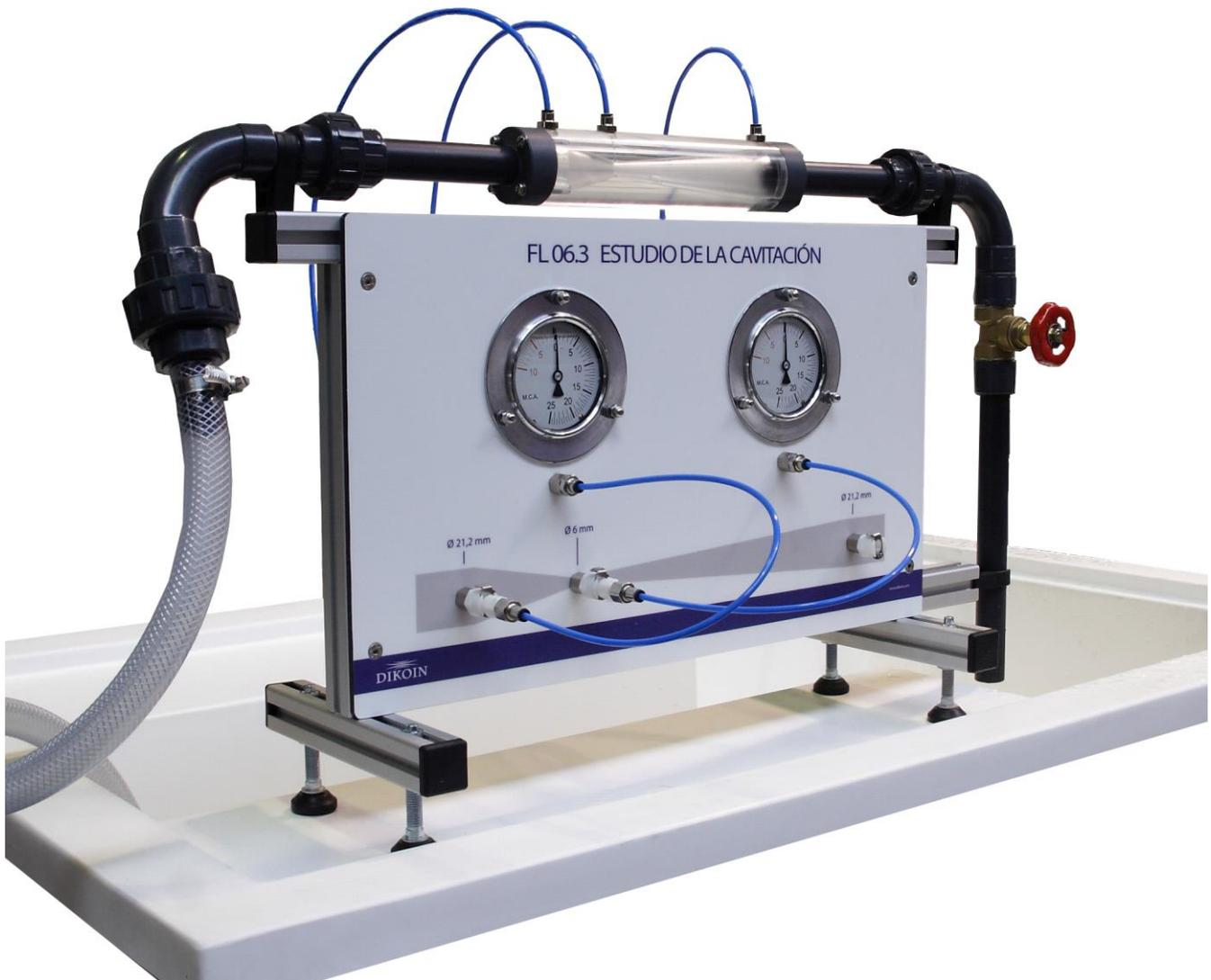
The demonstration equipment of the CAVITATION phenomenon is a simple equipment that is coupled to a hydraulic bench or any other source of hydraulic power supply.
